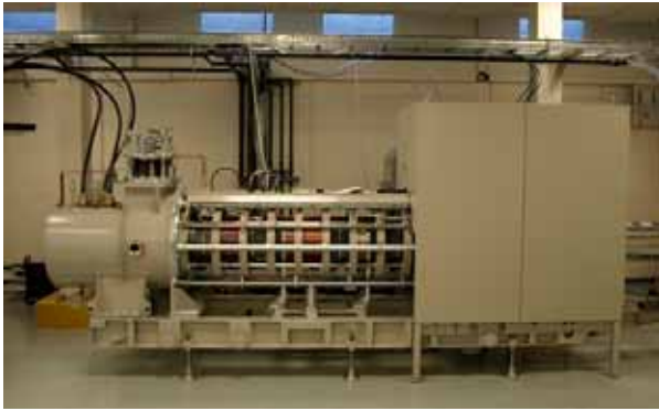
Figure 7. Toshiba klystron installed in the ISIS KPS Test Stand.
