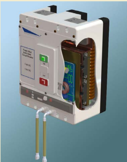
1 MW Solid-State DC Circuit Breaker. This molded-case circuit breaker operates at 1 kA and 1 kVDC. It maintains the look, functionality, and feel of a conventional 2.5 kA, 480 VAC three-phase circuit breaker.
