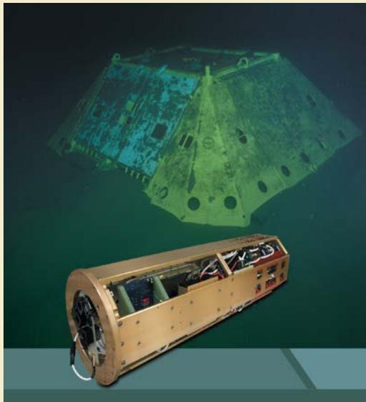
**Subsea MVDC Power Converter.** This 18" diameter pressurized module (foreground) resides within the Primary Node (background) at depths up to 3,500 meters. It converts 10 kVDC to 375 VDC directly on the seafloor for use by a wide range of specialized electronics.
