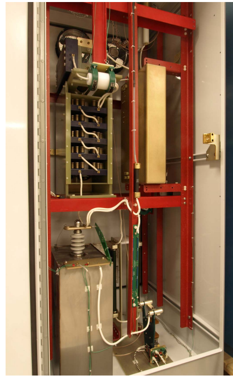
Figure 2. High-voltage cabinet for the pulsed amplifier. The modulator is at the middle left, and has blue switch plates. This cabinet is air-insulated.
