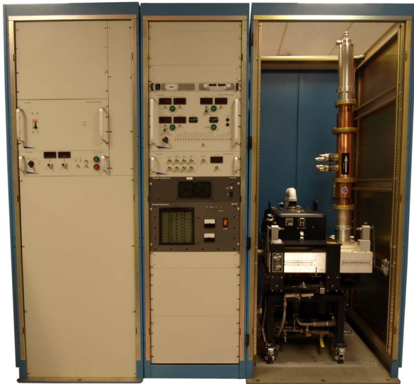
Figure 1. Modular multiple-frequency RF amplifier, CW version. The left cabinet holds the inverter, controls and tank for the HV power supply (behind a panel). The middle cabinet holds the solenoid supply, control box for faults and auxiliary supplies, RF metering, RF predriver, and RF driver. The right rack contains a 704 MHz IOT and cavity.
