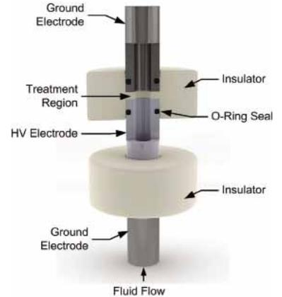
**Cutaway view of one-half of a PEF treatment chamber**, showing a single treatment zone. The pulsed electric field is applied to the fluid as it flows through the treatment zone.
