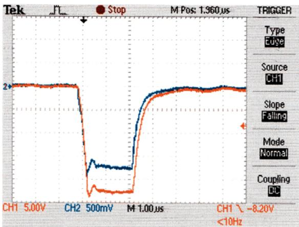
Figure 6. 20 kV, 35 A pulse into orange juice. Risetime ~ 200 ns, 1 kHz frequency
