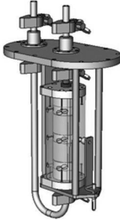
Figure 3. Cutaway drawing of 20 kV, 150 l/hr PEF treatment chamber.
