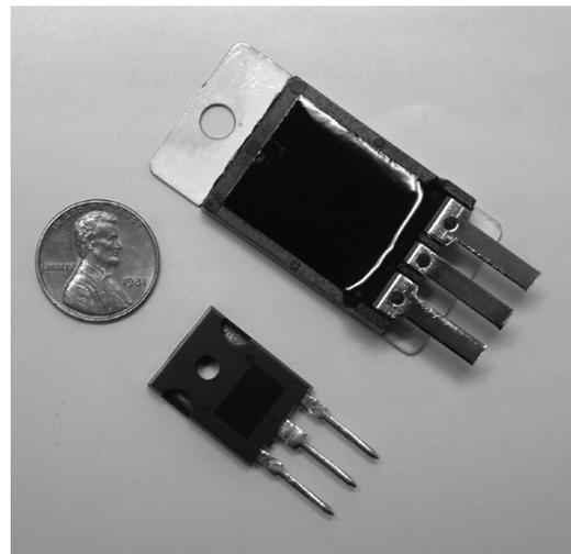
Figure 4. Pulse power transistor (PPT) top; conventional T0-247 bottom.
