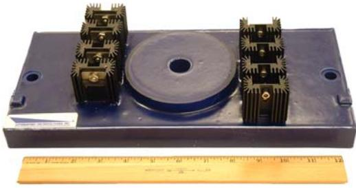
Figure 5. 20 kV, 100+ A, PPT switch module.
