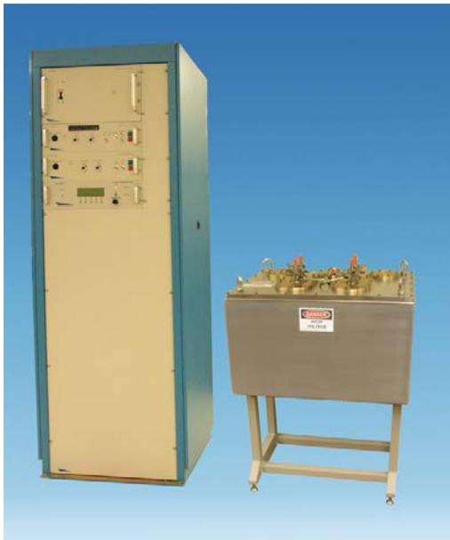
Figure 1. PEF pilot plant. Capacity up to 400 l/hr. Power electronics in cabinet on left; four-chamber processing unit on right.
