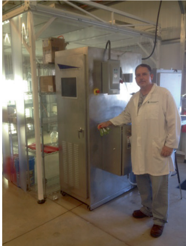
Fig. 2 Laboratory PEF System from Diversified Technologies, Inc. (DTI), installed at Arizona State University (ASU) in September 2014. This PEF system operates at up to 20 kV and 10 kW average power
