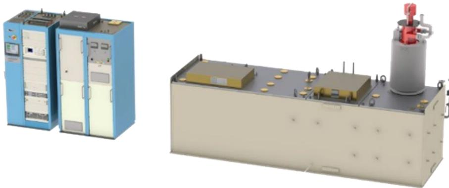
Fig. 1. 250 MW Peak Power CLARA Klystron Modulator System. High voltage solid-state switching allows a simple and reliable modulator with extremely high pulse fidelity and stability. One rack houses low voltage circuitry and controls (left) while a double-wide rack houses the standard high voltage power supply and step-up AC transformer (center), allowing standard US 480 VAC input to the HVPS from 380 VAC British power.
