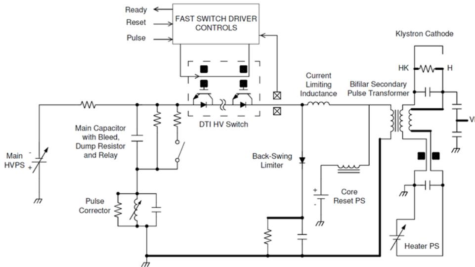
Fig. 2. Simplified modulator schematic. Directly switching 35 kV on the primary simplifies the pulse transformer and improves the risetime compared to higher step-up ratio designs. Series IGBT switches have inherent redundancy such that several modules may fail before system performance is affected.
