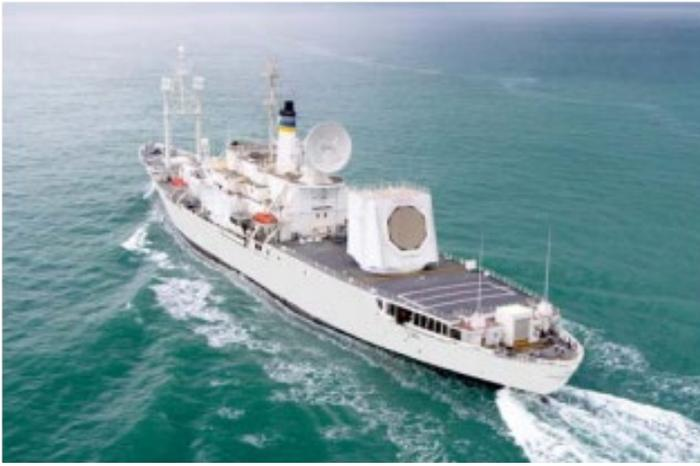
Figure 1. USNS Observation Island. The Cobra Judy Sband radar array is located aft of the Cobra Judy X-band dish.
