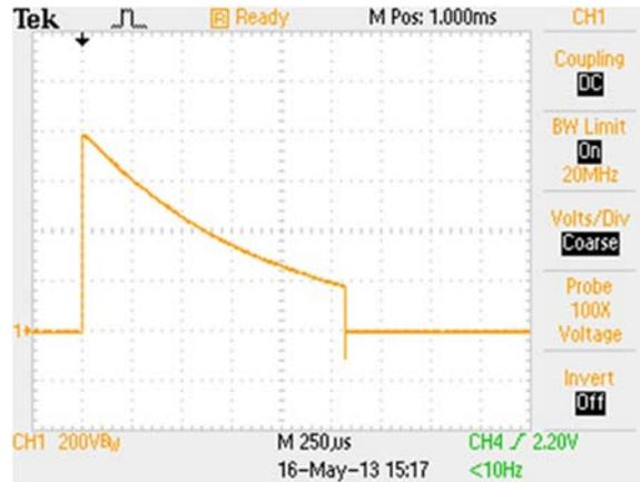
Figure. 1: Pulse voltage without the regulator, 200 V/div, 250  $\mu$ s/div.
