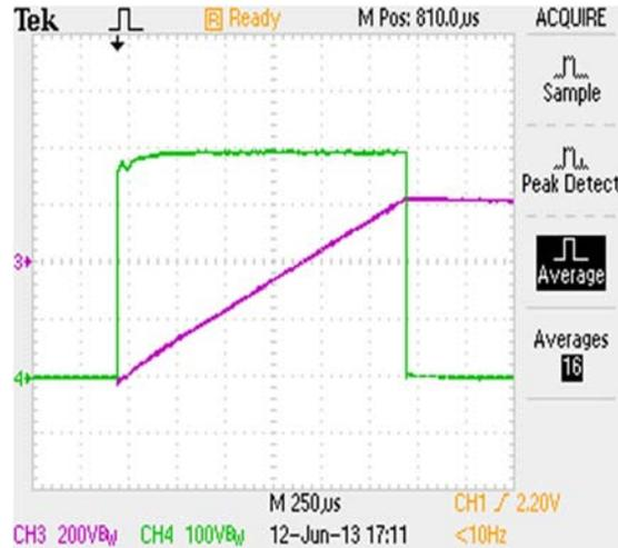
Figure. 2: Pulse voltage (green) and regulator voltage (purple) with the regulator, 200 V/div, 250  $\mu$ s/div.
