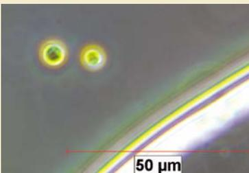
**Isocrysis algae PEF treated at DTI in 2009.** Top: Control (live) cells captured near a bubble (bottom-right of photo). Bottom: PEF-treated electroporated cells. Nine of eleven cells are clearly lysed in this view.
