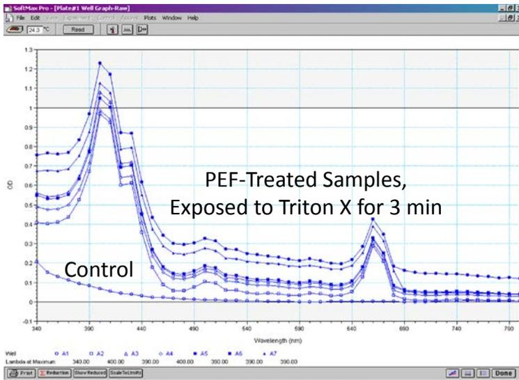
**Spectrophotometric wavelength scans illustrate the release of multiple pigments in Chlorella vulgaris after PEF treatment at different intensities. \*\***
