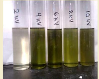
**Chlorella vulgaris samples after PEF treatment at different field strengths and centrifugation.** Spectrophotometric scans for pigment liberation showed clear differentiation as a function of PEF treatment, indicating that increased lysing of the algal cell membranes occurred at higher field strengths and pulse durations, releasing intracellular components into the supernatant.\*\*
