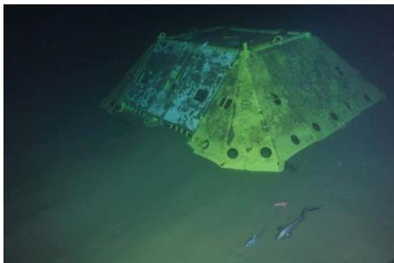
Figure 6. One of the seven primary MVPC nodes on the ocean floor.
