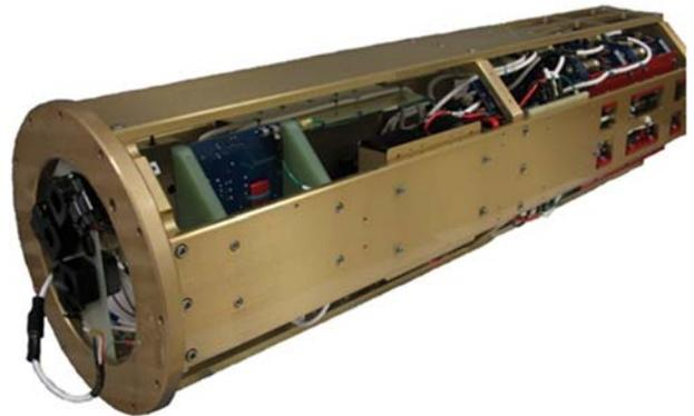
Figure 1. Undersea 10 kW Medium Voltage Power Converter (10 kV to 375 V). These are located in 3km of water 900km from shore.
