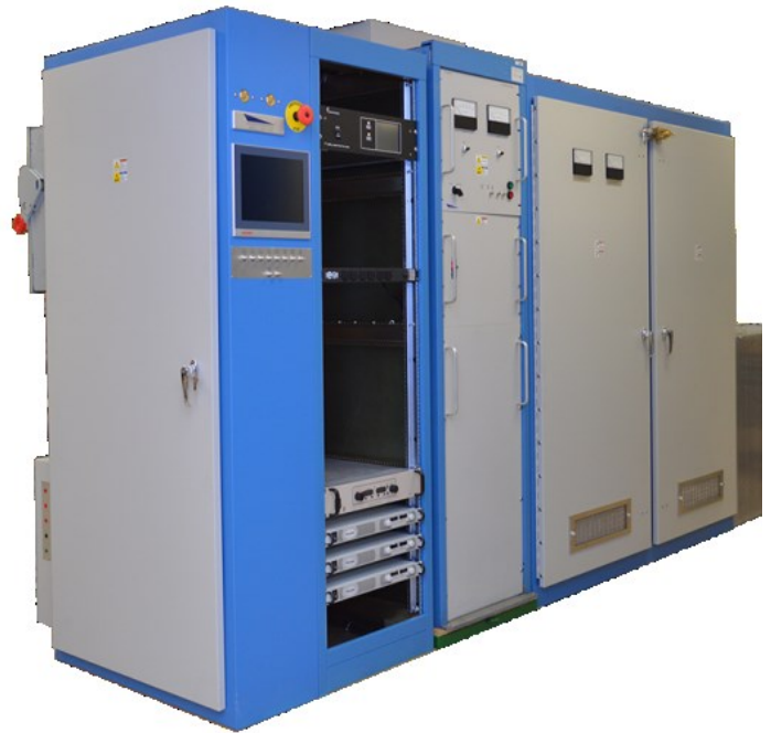
Fig. 1. Complete Klystron Test Stand, showing controls and auxiliary supplies in the left cabinet (Cabirack), the high voltage power supply (center-left), the high voltage modulator cabinets (center-right), and stand (right).
