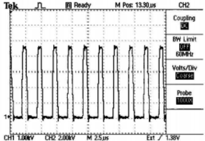
Figure 7: 4.5kV, 400kHz pulse
