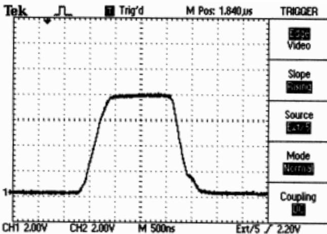
Figure 5: Transmitter pulse 8kV, 100kHz, 1.5µs
