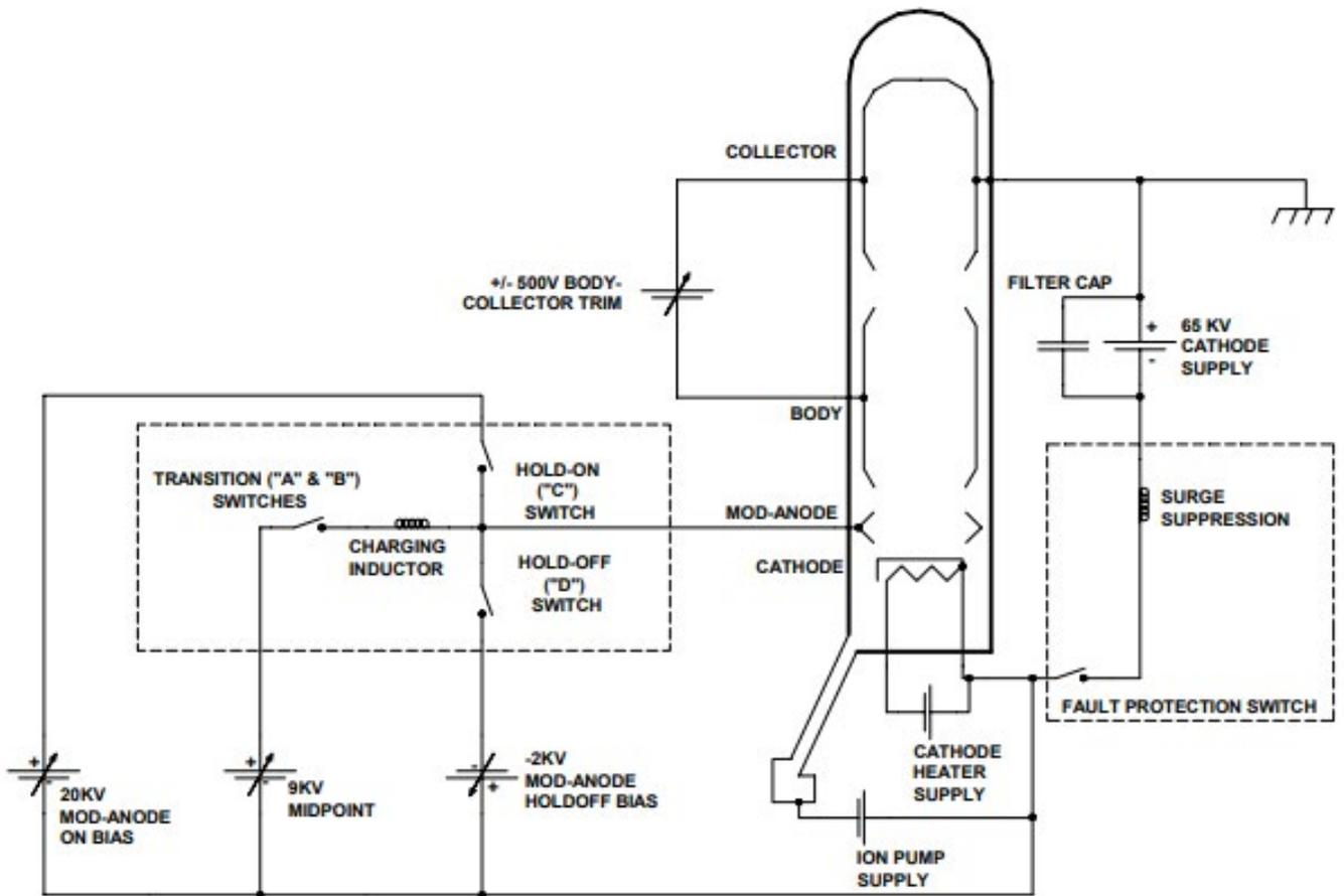
Figure 8: Schematic of NRL gyrokystron modulator.
