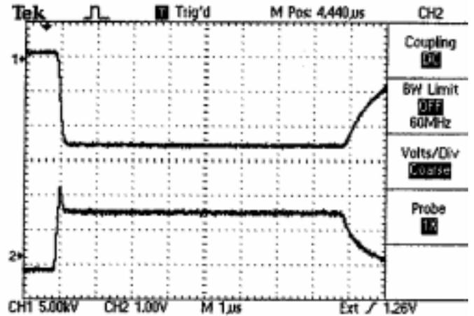
Figure 6: AN/SPG-60 Pulse, 13.5kV, 25 kHz, 8 µs
